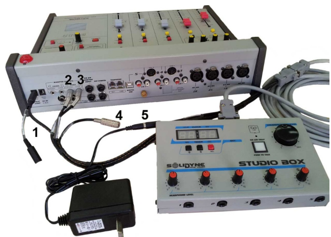
Figure 2: The DB9 connector was replaced by RJ45 in new models ternal power source 110/220V 1.25A.
